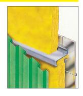
sheeting. Spacer bars of non compressible material should be used to prevent undue crushing of the insulation.
